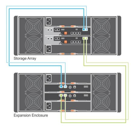
Figure 5. Single expansion diagram
